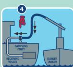
4 Ensure sampling starts simultaneously with the bunkering operation.
